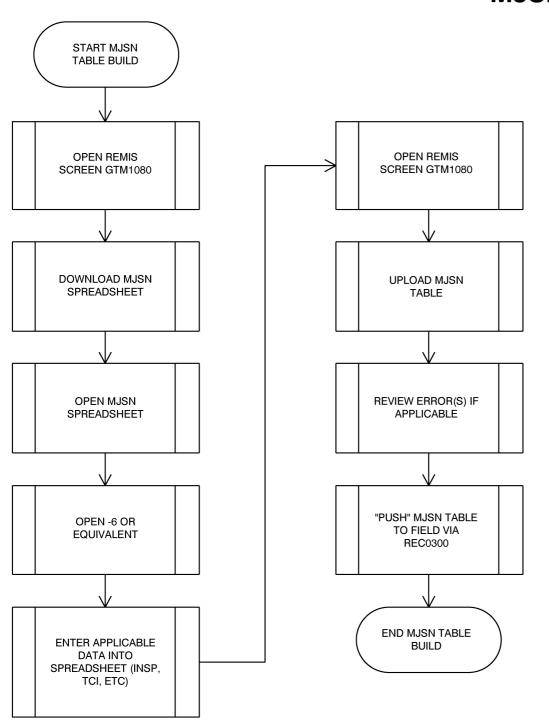
Figure 6-1. MJSN Process Flow Diagram - Build
