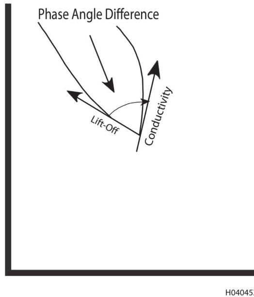
Figure 4-15. Phase Angle Difference between Lift-Off and Conductivity
