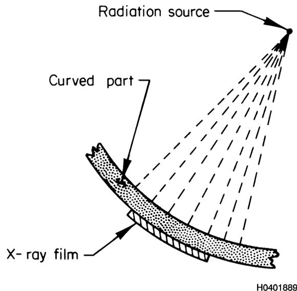
**Figure 6-25. Preferred Geometry for Radiography of Curved Surfaces**
