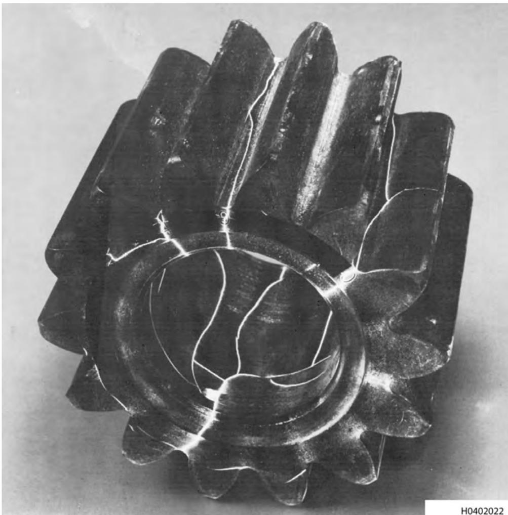
**Figure 3-41. Typical Magnetic Particle Indications of Cracks**
