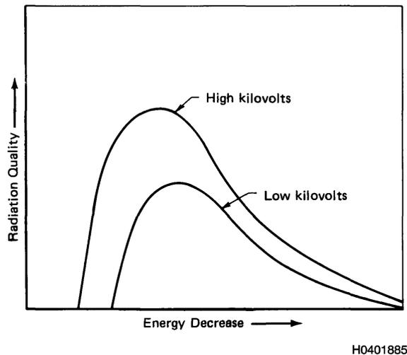
Figure 6-21. Effect of Kilovoltage on Transmitted Radiation Output
