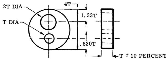
DESIGN FOR PENETRATOR THICKNESSES OF 0.180 AND OVER MADE IN .020 INCREMENTS
