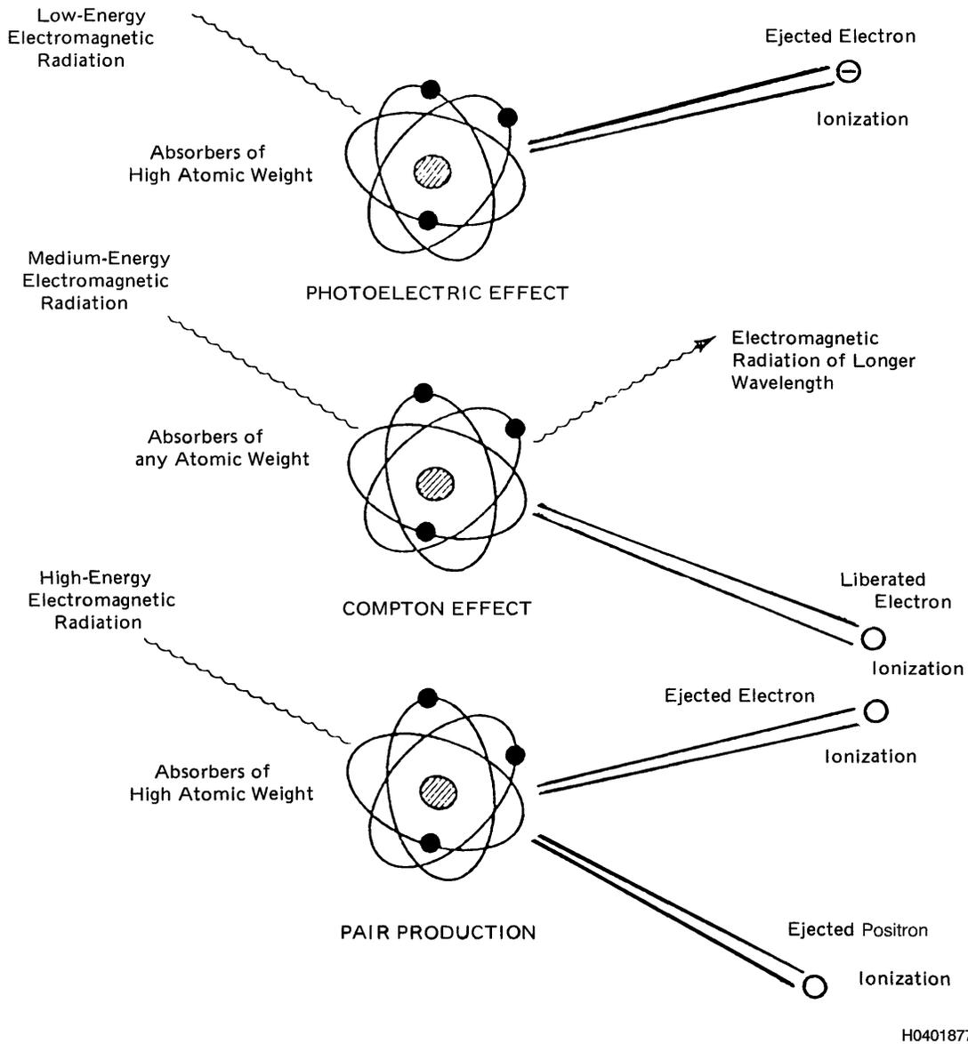
**Figure 6-13. Illustration of Various Radiation Absorption Interactions**
