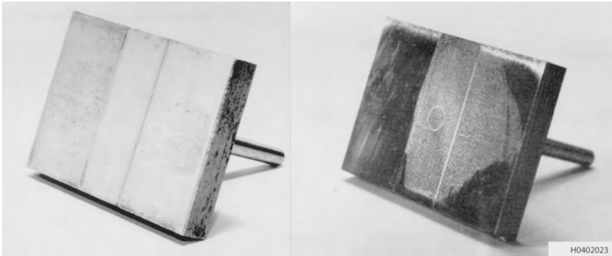
**Figure 3-42. Magnetic Particle Indication of a Forced Fit**
