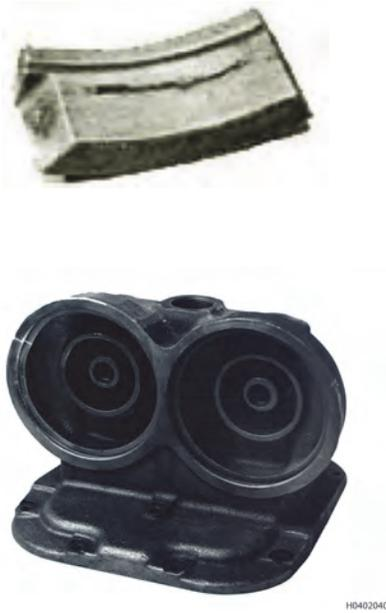
**Figure 3-59. Magnetic Particle Indications of Defects in Castings**
