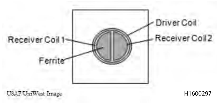
**Figure 4-34. Coil Configuration in a Bolt Hole Probe**
