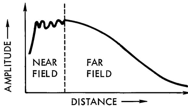
**Figure 5-9. Amplitude Response Curve of Typical Transducer**
