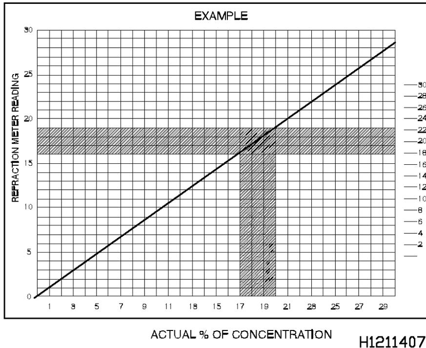
**Figure 2-36. Remover Concentration vs Refractive Index Graph**
