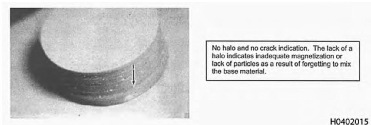
Figure 3-34. Magnetic Rubber Replica With No Indication
