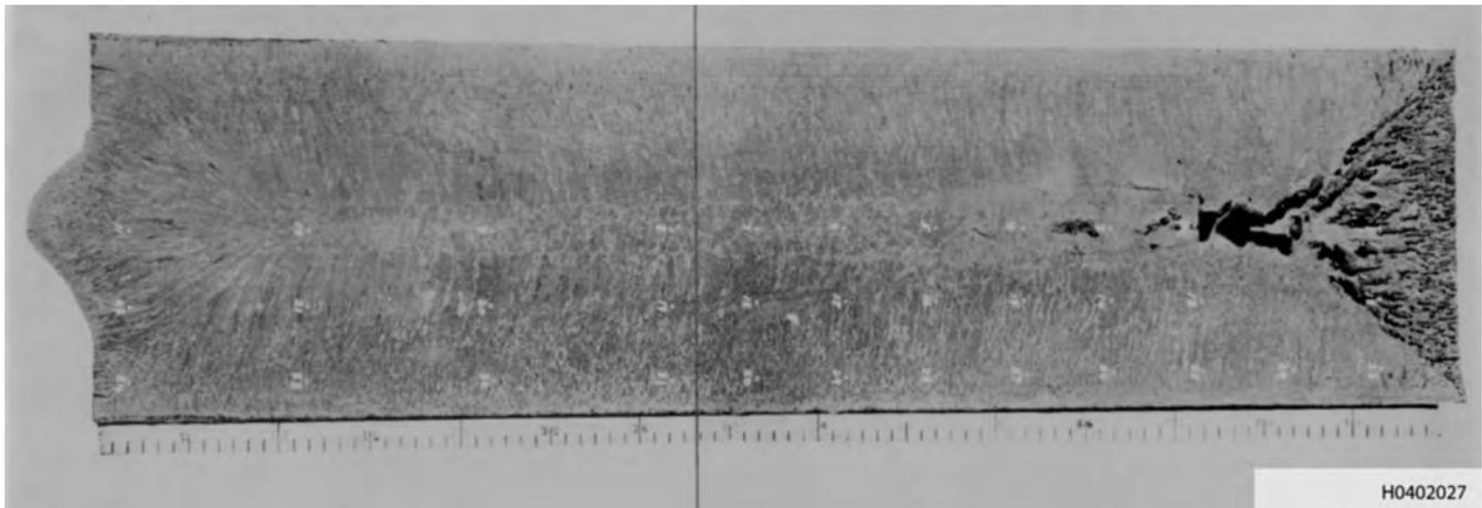
**Figure 3-46. Cross-Section of Ingot Showing Shrink Cavity**
