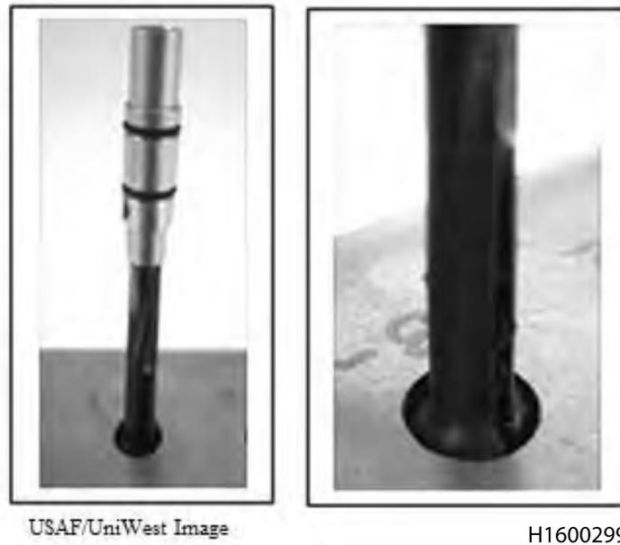
**Figure 4-36. Checking Probe Fit**
