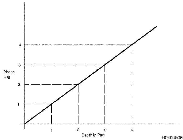
**Figure 4-23. Phase Lag and Depth in Part**
