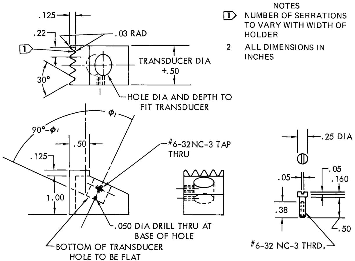
Figure 5-28. Angle Beam Wedge With Hole for Mounting Transducer
