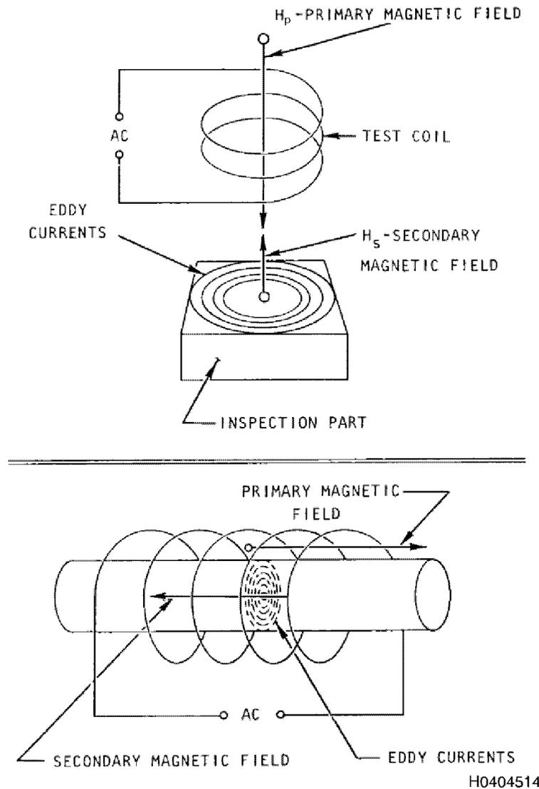
Figure 4-6. Primary and Secondary Magnetic Fields in ET
