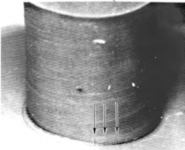
Corner cracks ranging in size from 0.002" to 0.015".
