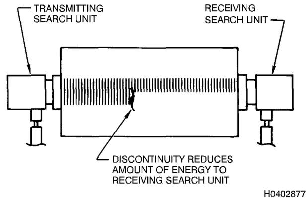
**Figure 5-43. Through-Transmission Inspection**
