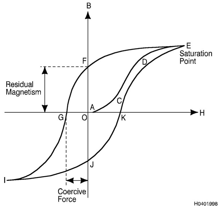
Figure 3-17. Hysteresis Curve for a Ferromagnetic Material
