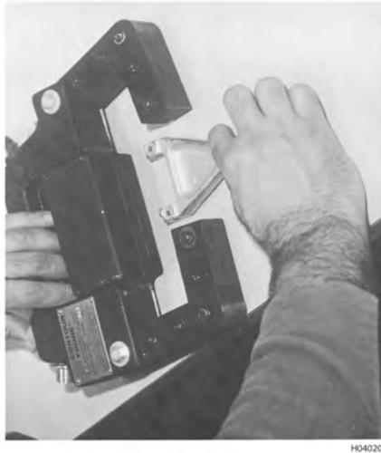
**Figure 3-31. Non-Contact Demagnetization**
