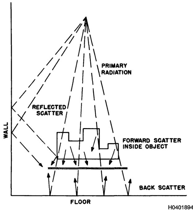
Figure 6-28. Sources of Scatter Radiation
