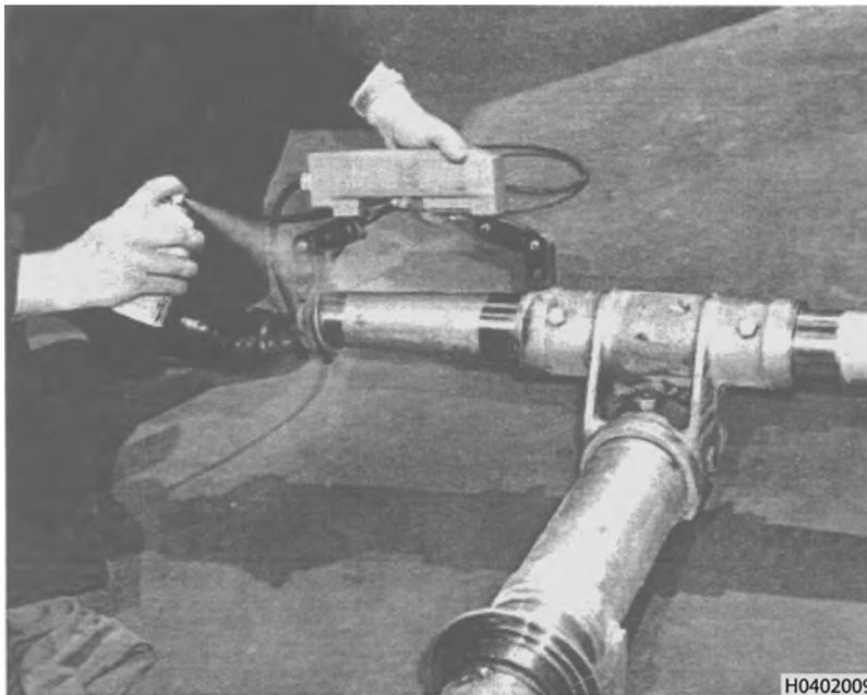
**Figure 3-28. Field Inspection of Nose Wheel Strut**
