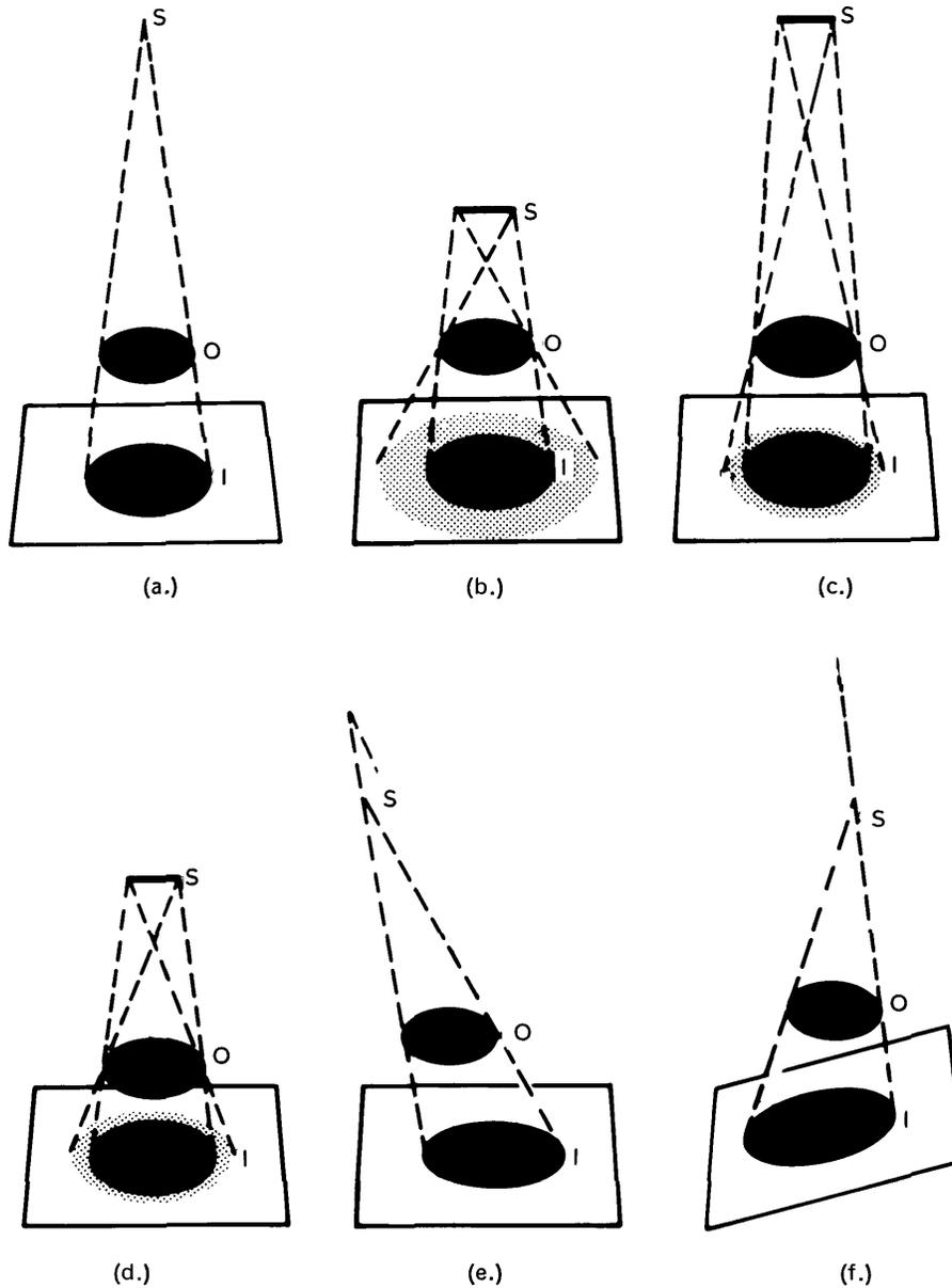
S REPRESENTS THE SOURCE, O REPRESENTS THE OBJECT BEING RADIOGRAPHED, AND I IS THE IMAGE PLANE. (a) OPTIMUM GEOMETRIC FIDELITY CONDITION. (b) EFFECT OF POOR  $F/d$  RATIO WITH LARGE PENUMBRA SHADOW, (c) CONDITION IMPROVED BY INCREASING SOURCE-TO-OBJECT DISTANCE. (d) SAME CONDITION ACHIEVED BY DECREASING PART THICKNESS OR DISTANCE FROM OBJECT TO FILM. (e) AND (f) ILLUSTRATE THE EFFECT OF GEOMETRICAL MISALIGNMENT.
