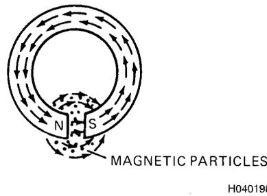
Figure 3-2. Horseshoe Magnet With Poles Close Together
