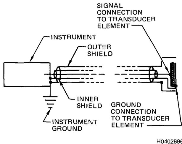
**Figure 5-59. Double Shield for Reducing External Noise Signals**
