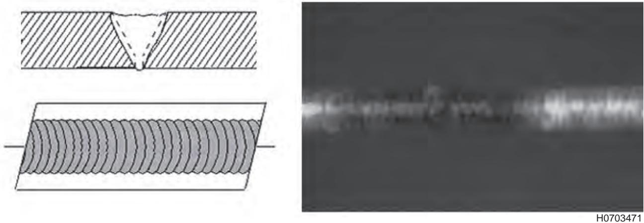
**Figure 6-57. Inadequate Weld Reinforcement**
