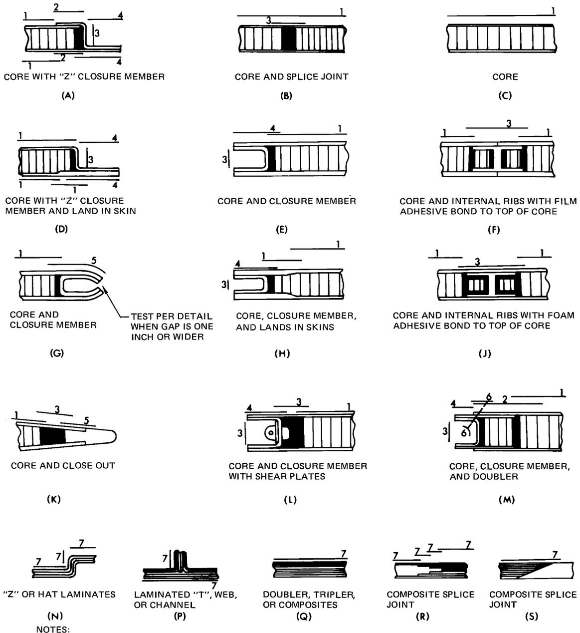
1. THE NUMBERED LINES SURROUNDING EACH VIEW INDICATE THE SCAN PLANES. THE NUMBER ON EACH LINE IS USED TO DETERMINE THE ACCEPTABLE INSPECTION METHODS BY REFERRING TO TABLE 5-1.
