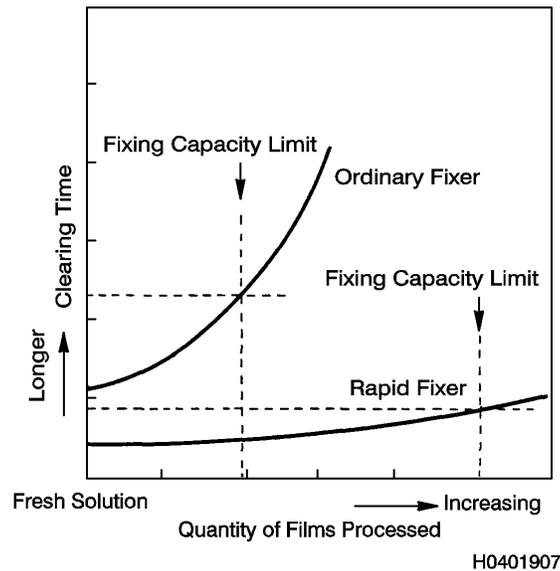
Figure 6-40. Clearing Time and Fixing Capacity of Fixers
