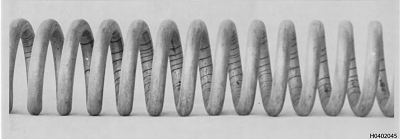
**Figure 3-63. Magnetic Particle Indications of Plating Cracks**
