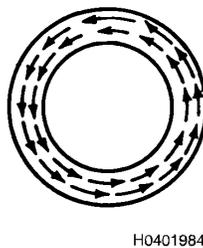
Figure 3-3. Horseshoe Magnet Fused Into a Ring
