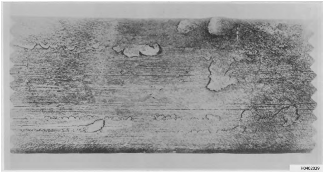
Figure 3-48. Scabs on the Surface of a Rolled Bloom
