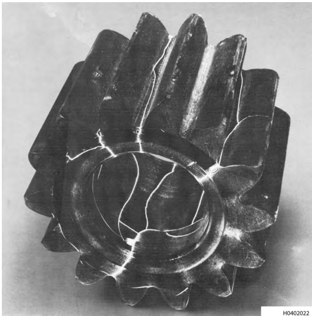
Figure 3-41. Typical Magnetic Particle Indications of Cracks
