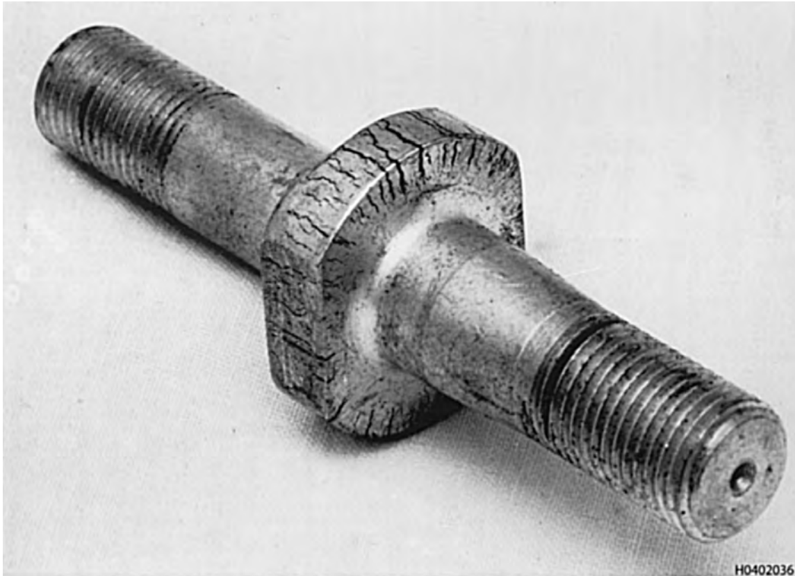
Figure 3-55. Magnetic Particle Indications of Forging Cracks or Bursts in an Upset Section, Severe Case
