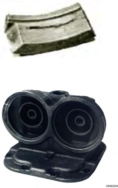
Figure 3-59. Magnetic Particle Indications of Defects in Castings
